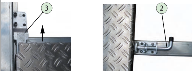
Sliding the drive-up ramps in
