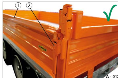
**Fig. 13** Drop-side, secured
