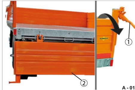
**Fig. 20** Rear platform gate folded down
