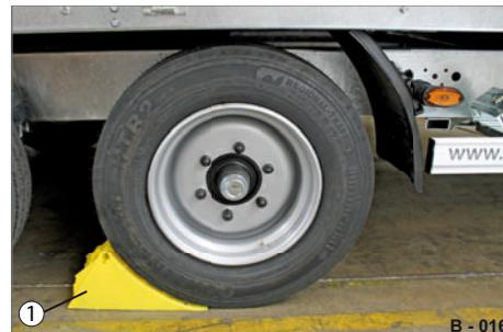
**Fig. 21** Wheel chocks positioned
