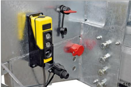
Fig. 14 Pushbuttons and main switch for tipping operation I - 016
