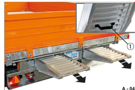
**Fig. 51** Pulling out the ramps
