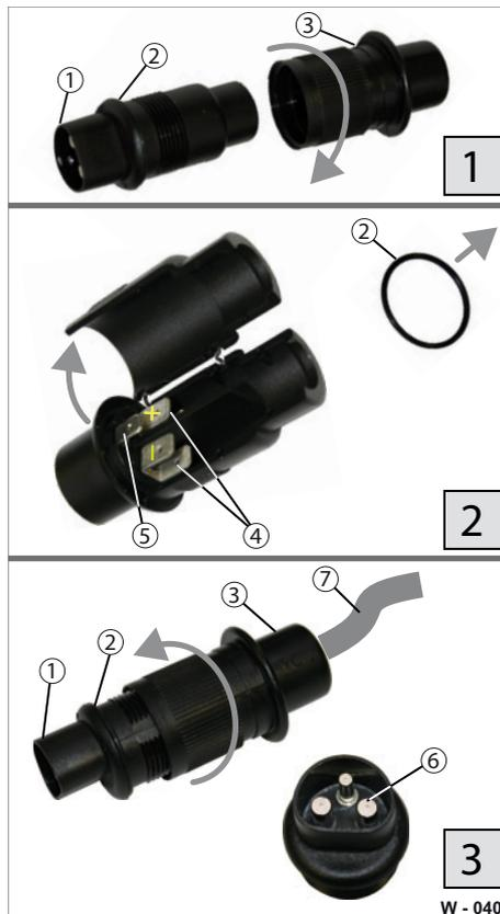
Fig. 33 Charging plug for charging device
