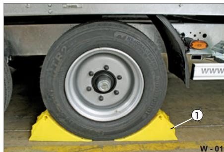
**Fig. 37** Securing the vehicle
