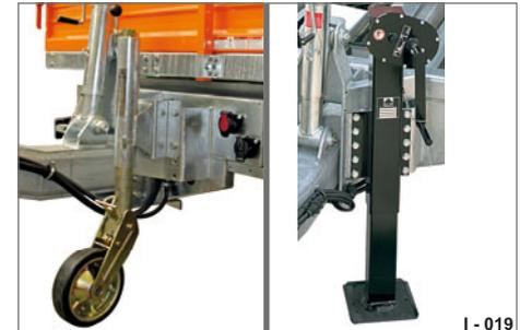
Fig. 20 Support equipment on the draw bar
