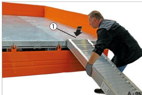
**Fig. 56** Putting the ramps in position
