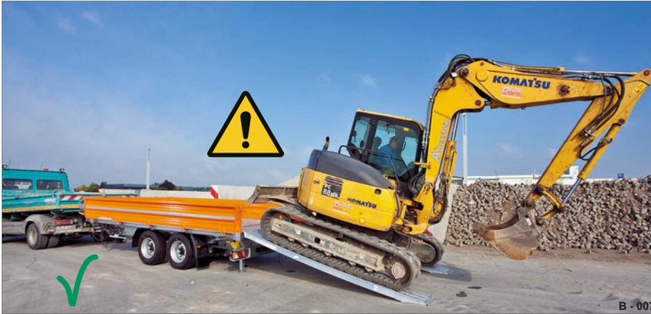
Fig. 4 Driving onto the trailer
