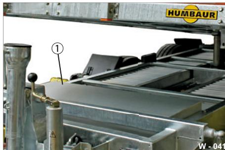
**Fig. 30** Electro-hydraulic unit, closed
