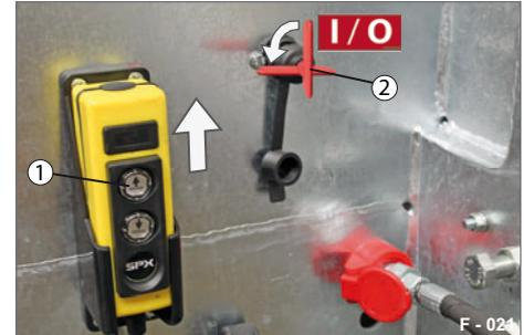
**Fig. 34** Tipping the loading platform
