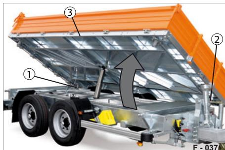
**Fig. 49** Loading platform tipped to the side
