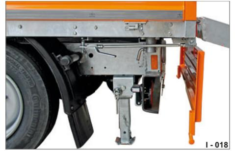
Fig. 25 Folding supports on the rear
