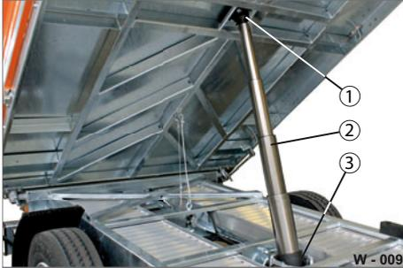
**Fig. 26** Checking / servicing the cylinder
