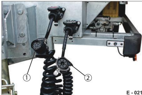
**Fig. 4** Connection cables 12 V / 24 V
