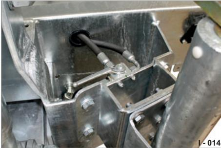
Fig. 15 Switch lever, hydraulic supply
