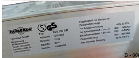
Fig. 5 Name plate, ramps
