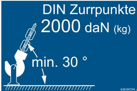
Fig. 65 Example of a lashing point label
