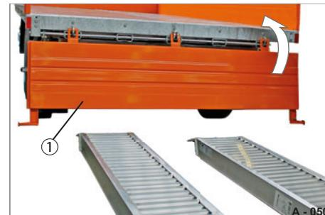
**Fig. 60** Closing the rear platform gate
