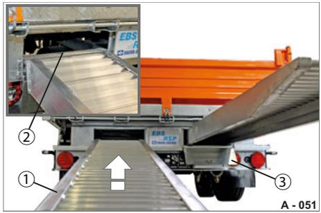
**Fig. 61** Sliding the ramps in
