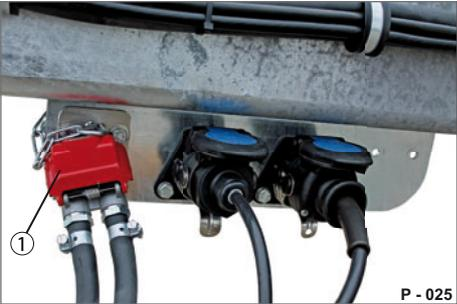
Fig. 6 Duo-Matic quick-release coupling system
