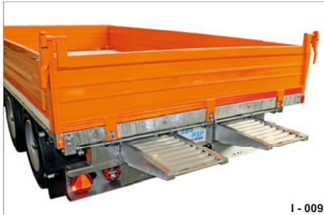
Fig. 9 Ramp stowage compartments in the chassis I - 009
