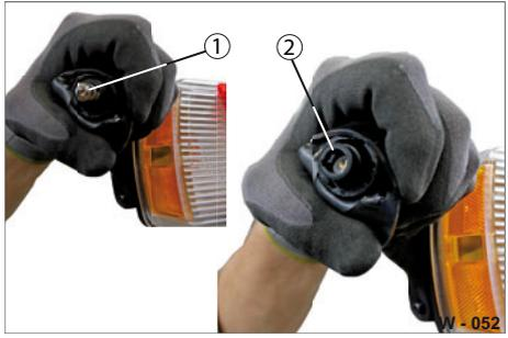
**Fig. 51** Replacing the lamp
