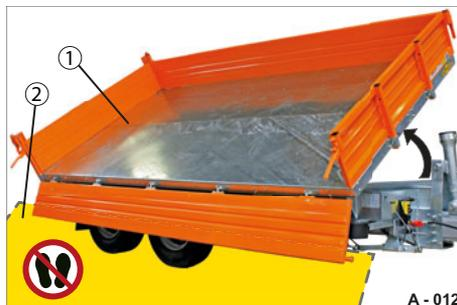
**Fig. 12** Loading platform tipped to the side
