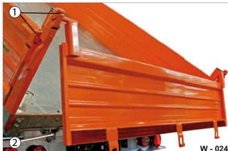
**Fig. 14** Lubrication points
