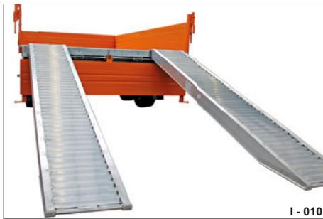
Fig. 10 Rear platform gate, folded down I - 010
