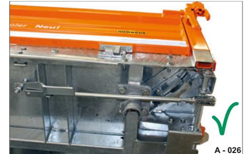
**Fig. 27** Central interlock, closed
