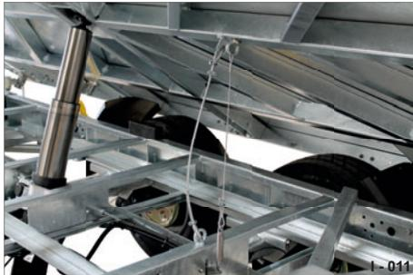
Fig. 11 Loading bridge tipped to the side I - 011
