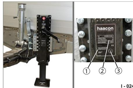
**Fig. 29** Spindle support (example)
