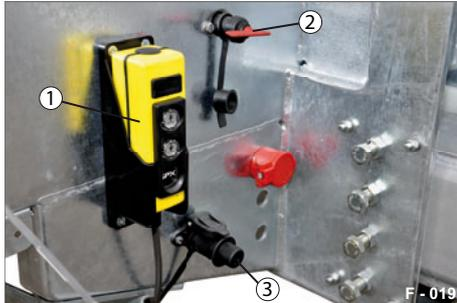
**Fig. 32** Electro-hydraulics control point
